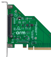
Figure 2-15: DSTREAM-XT x8 card edge adapter
