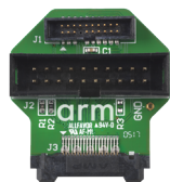
Figure 2-12: MICTOR 38-way 4-bit adapter
