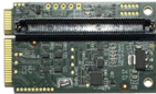
Figure 2-17: Mini-PCIe adapter
