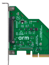
Figure 2-14: DSTREAM-XT x4 card edge adapter
